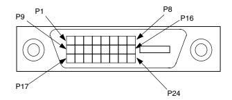
Figure H-6. DVI-D Monitor Connector (24-Pin Connector)
